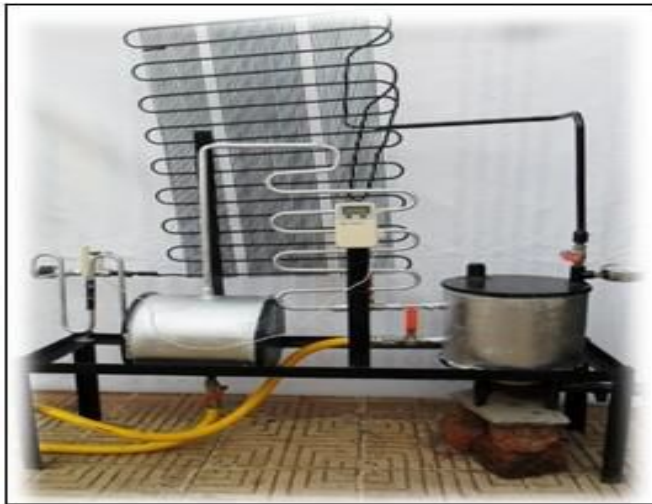
Fig.2 Complete view of vapour absorption refrigeration system.
